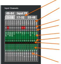
**Input Channels view** Tabs let you access all 64 input channels and the FX short returns.
